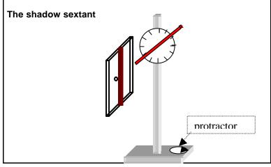
Measurement of the height angle of the sun
