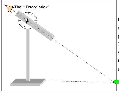
You make the stick turn until the view line (alidade) is aligned with the point to locate, then you fix the stick in that position.
