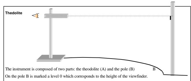
It needs two persons to be used. The pole is vertically laid upon the ground where you want to evaluate the difference of level with the one of the theodolite.
