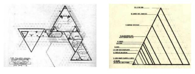
(a) (b) Figure 5 The plan of Palmer house (a) the self similar triangles inside the Palmer house (b).
