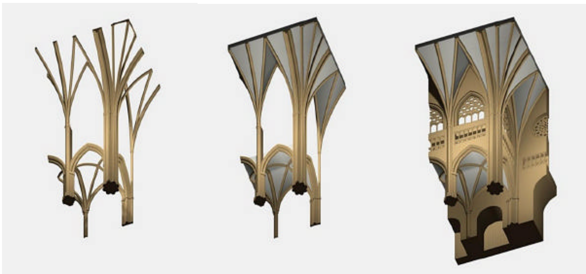
Fig 4. Interior of the Bilbao Cathedral. The making of a computer model is similar to the physical creation of the Cathedral. First, the columns and arches are constructed, then the vaults, piers and flying buttresses and finally the walls, windows and ornaments.
