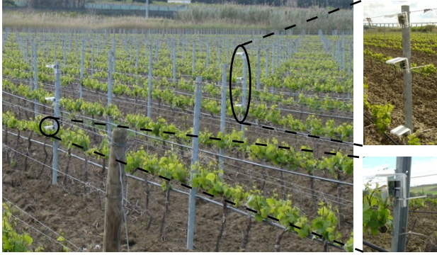
Figure 2. The WSN deployment in the vineyard.
