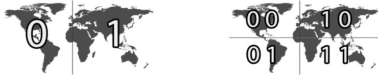
Figure 2. An example of how the first two bits of a geohash string are generated.
