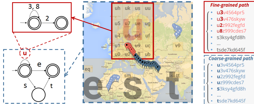
Figure 3. Given the DFA for a larger cell (dashed-line box), a more detailed model can be built by inferring the DFA for transition u (solid-line box).
