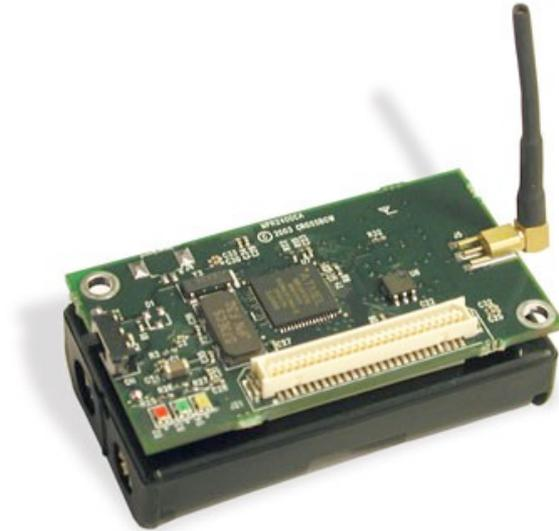
Figure 8.1: Crossbow MICAz mote.
