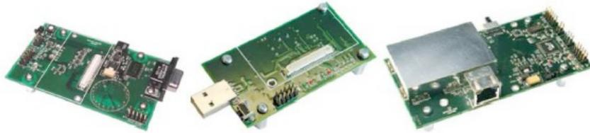
Figure 8.3: MIB510, MIB520 and MIB600 boards.
